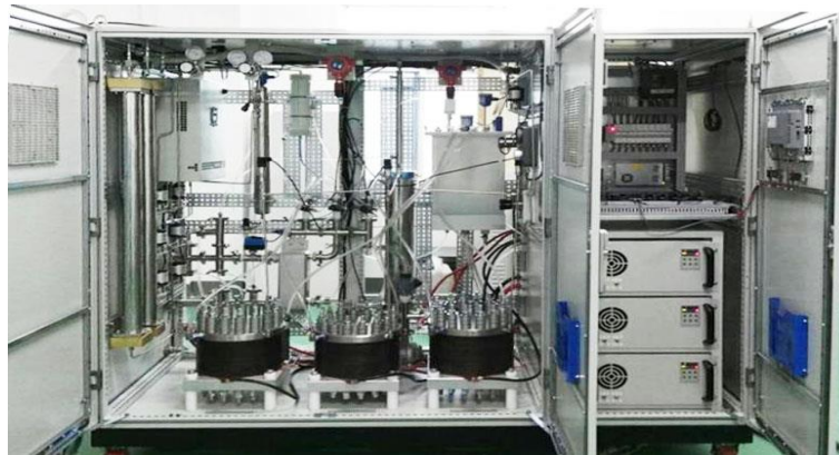
Figure 5.8. Equipment of 200 Nm 3 /h (1 MW) PEM (size: 2400*1700*2000)
